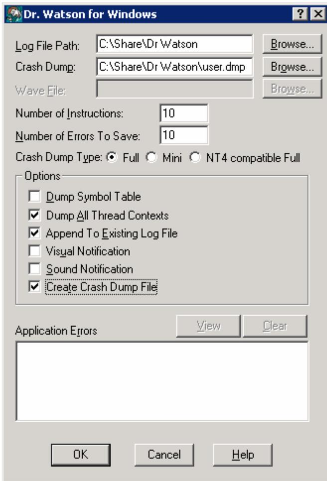
Typical setup of C:\Windows\system32\drwtsn32.exe to save a memory dump upon an application crash. Copy dmp file and
