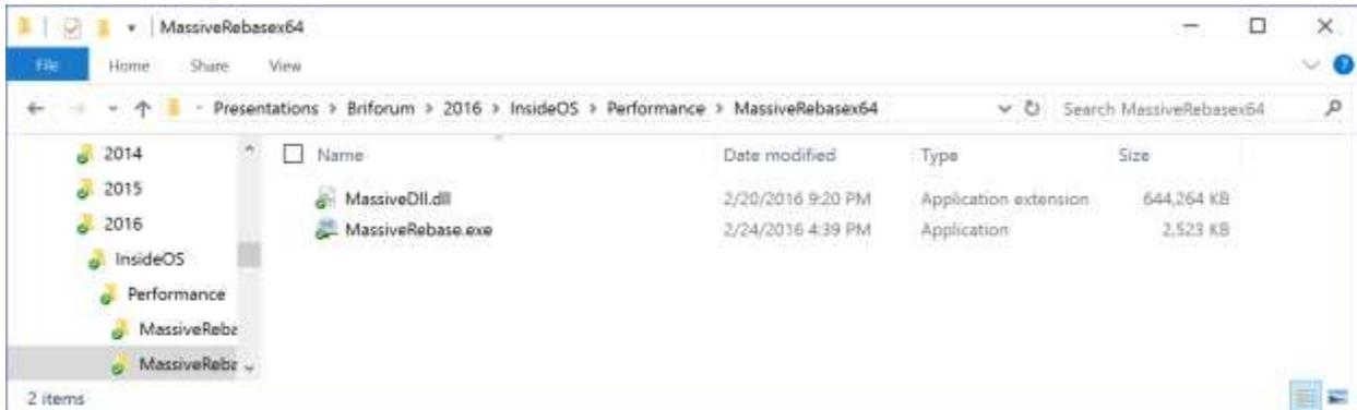
The dll created from the 25 million lines of code is 629MB, which works out to 26bytes per line of source code.
